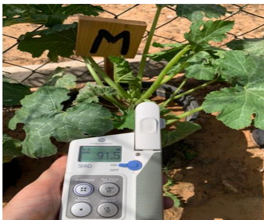
Fig. 2. Device used to estimate chlorophyll content in plant leaves.
